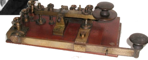
Marconi spark key used on Titanic
